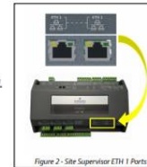
Figure 2 - Site Supervisor ETH 1 Ports
