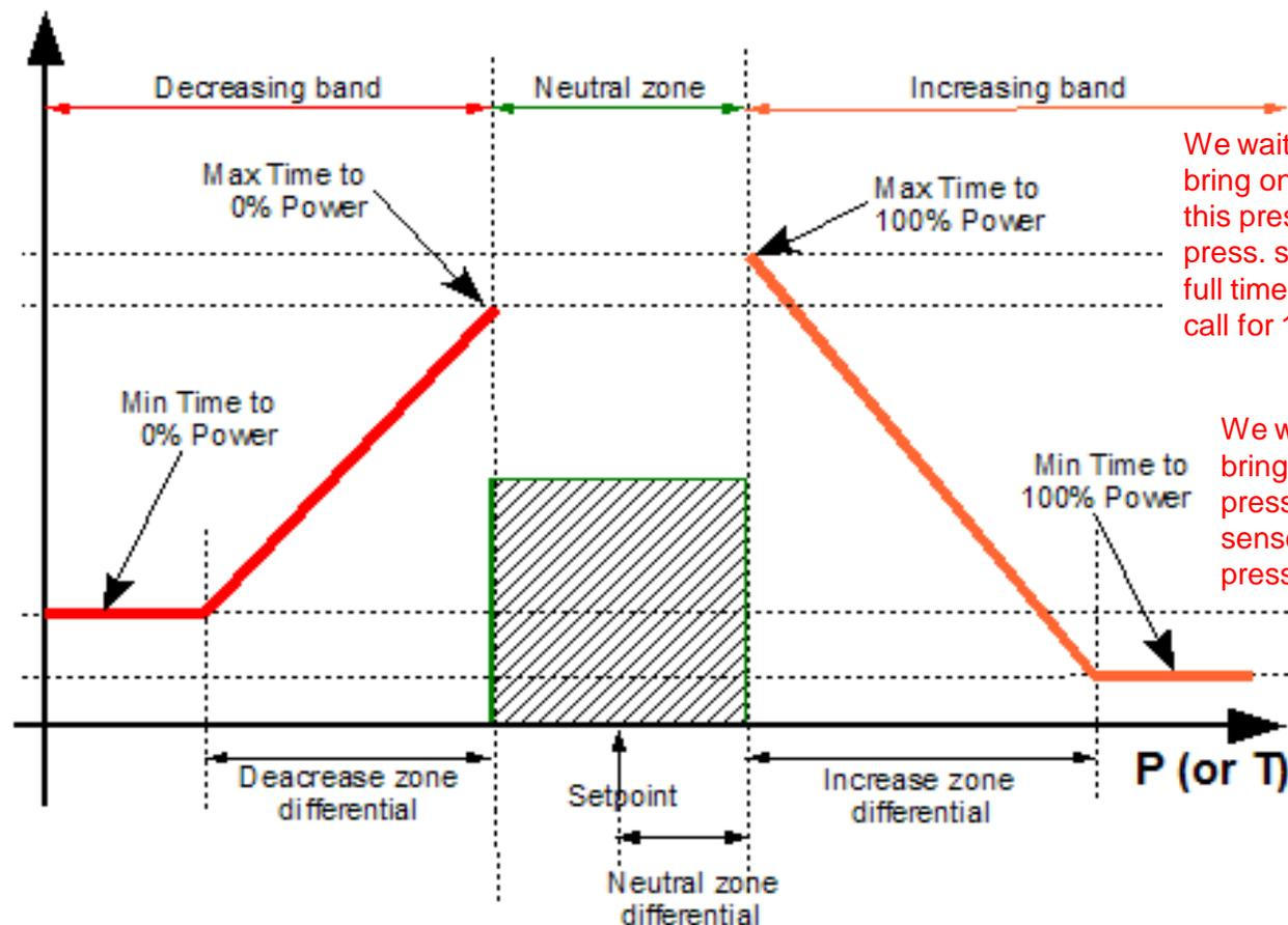
We wait the Max time to bring on 100% capacity at this pressure. So if the press. sits here, we wait the full time before we go to a call for 100% capacity.
