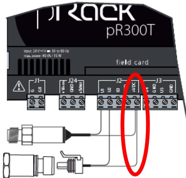
DO NOT CONNECT GREEN WIRE; CAP OFF. **Power from +VDC terminal**
