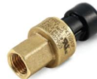
MT Discharge pressure: (SPKT00D8C0), 0-150 bar, 0-2175 psig, **4 – 20ma**, Gas 1/4 MPT (straight thread, o-ring included)
