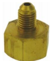
Thread Adapter All flammable refrigerant cylinders are left-threaded!
